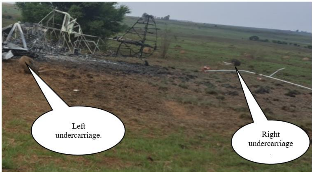
Figure 4: The left and the right landing gears at the accident site.
