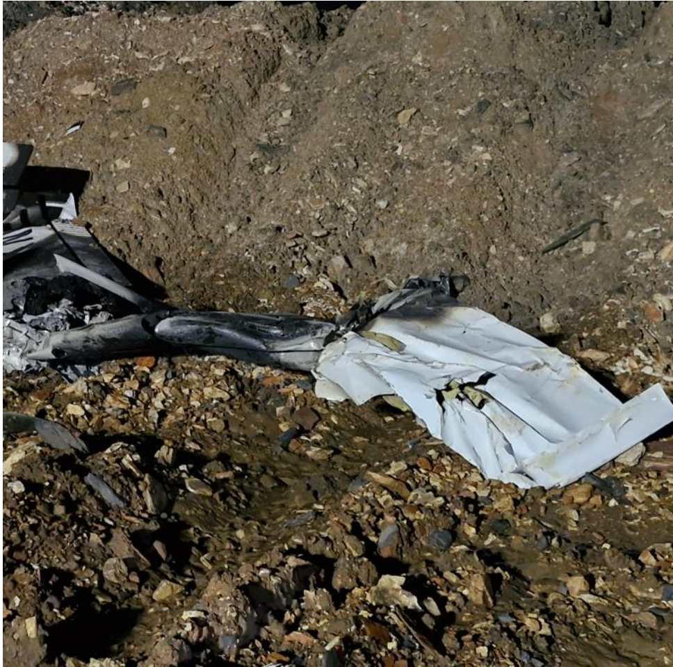
Figure 6: The deformed right wing.
