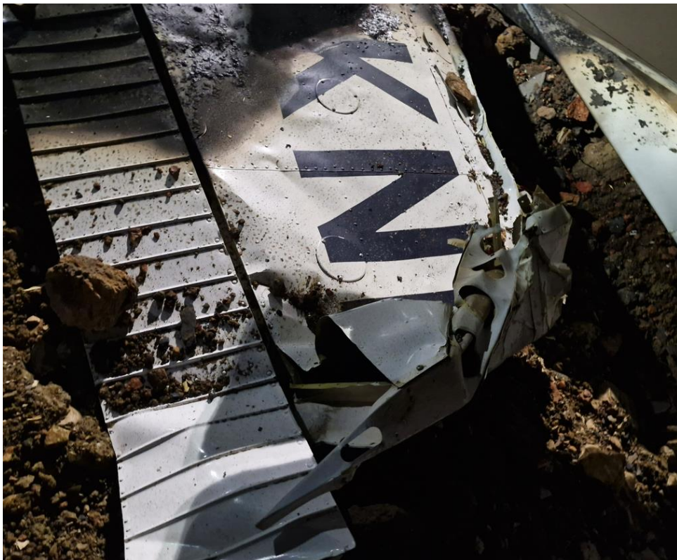
Figure 5: The deformed left-wing tip and aileron.
