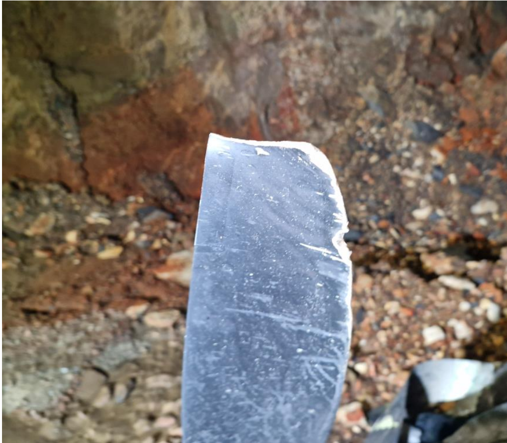
Figure 8: The damaged leading-edge tip.
