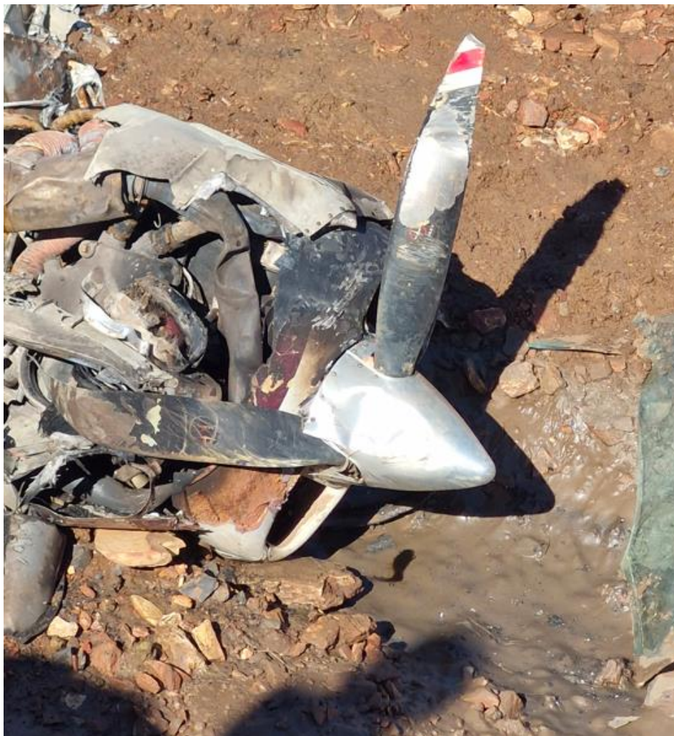
Figure 7: Damaged propeller blades.
