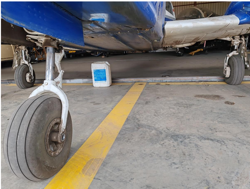
Figure 4: Scrape marks on the underbelly.
