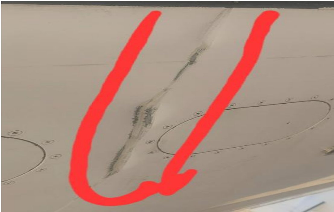
Figure 3: Damage on the underside of the right-wing tip.
