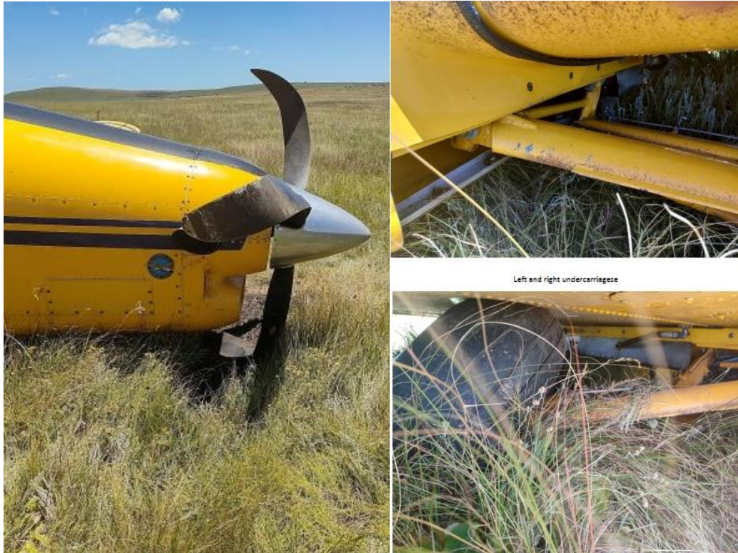
Figure 5: The pictures above depict the propeller and main undercarriage damage. (Source: Operator)
