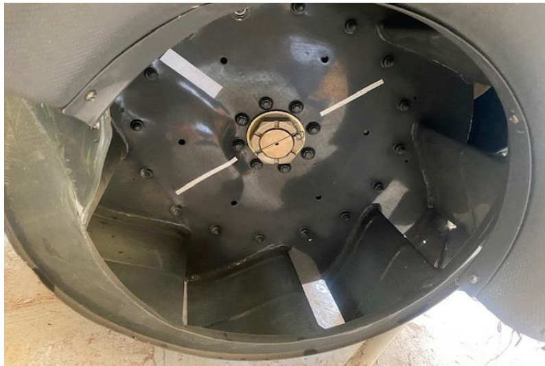
Figure 8: The engine cooling fan.
