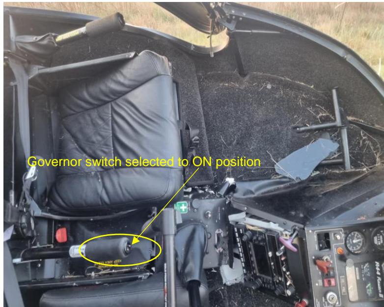
Figure 6: The pilot's collective pitch control stick in the UP position and the governor switch in the ON position.
