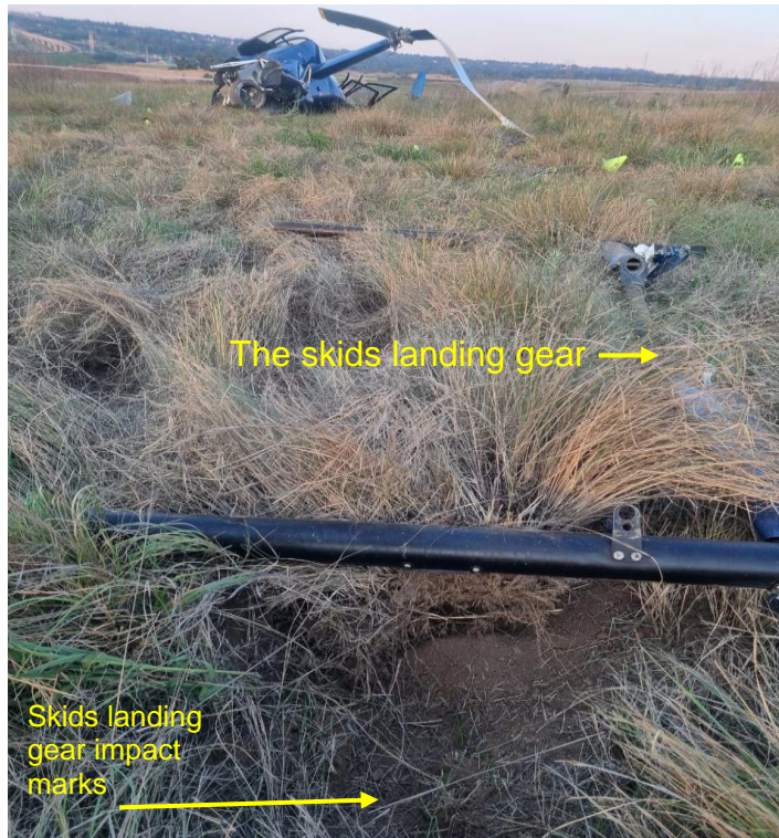
Figure 4: The wreckage and the broken skids landing gear.
