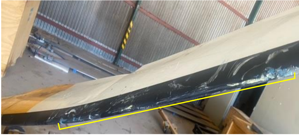
Figure 7: The main rotor blade leading edge area showing the impact print.
