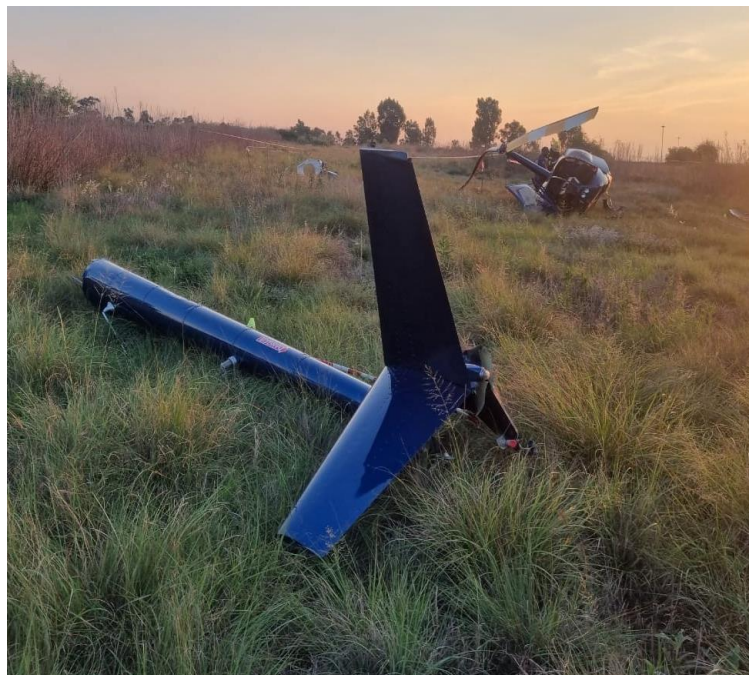
Figure 5: The main wreckage and the severed tail boom.
