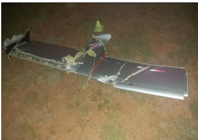
Figure 9: The severed horizontal stabiliser.
