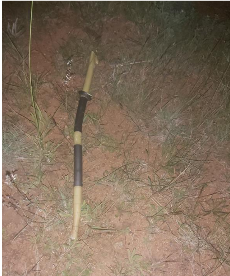
Figure 10: A section of the tail rotor drive shaft at the accident site.
