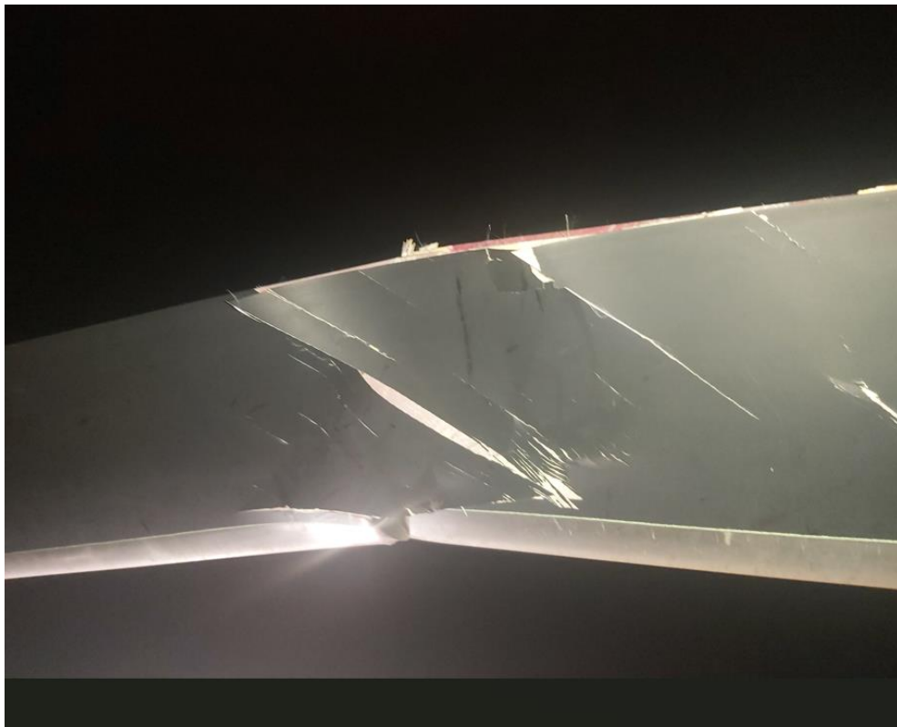
Figure 7: Damage sustained to one of the main rotor blades.
