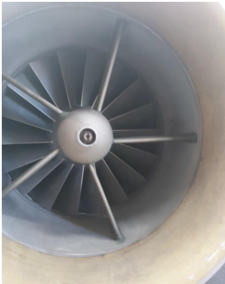
Figure 12: The undamaged engine inlet compressor blades.
