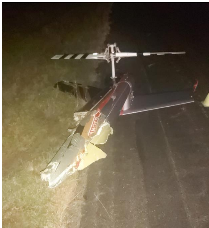
Figure 8: The tail cone at the accident site.
