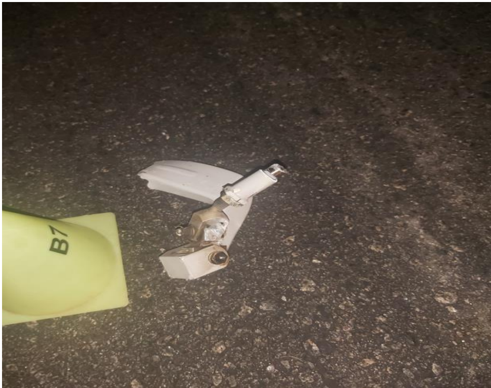
Figure 6: The damaged pitch change link attachment.
