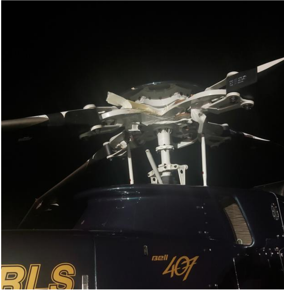
Figure 5: Damage to the main rotor head.
