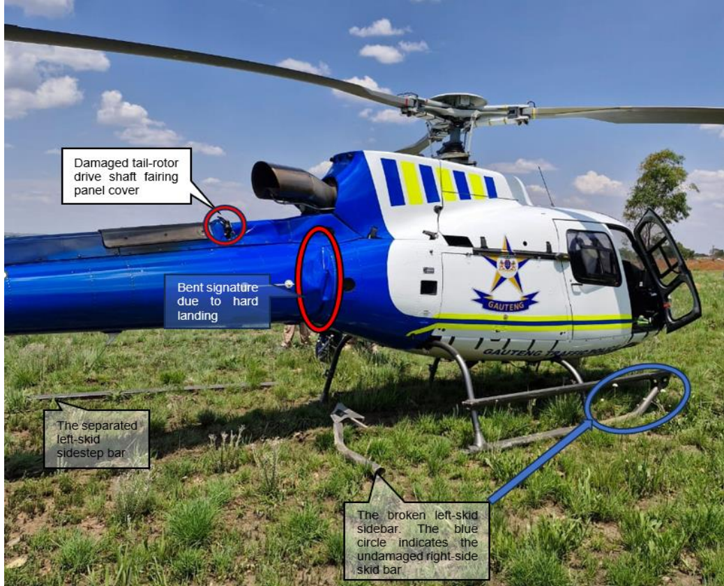
Figure 3: The helicopter post-accident.
