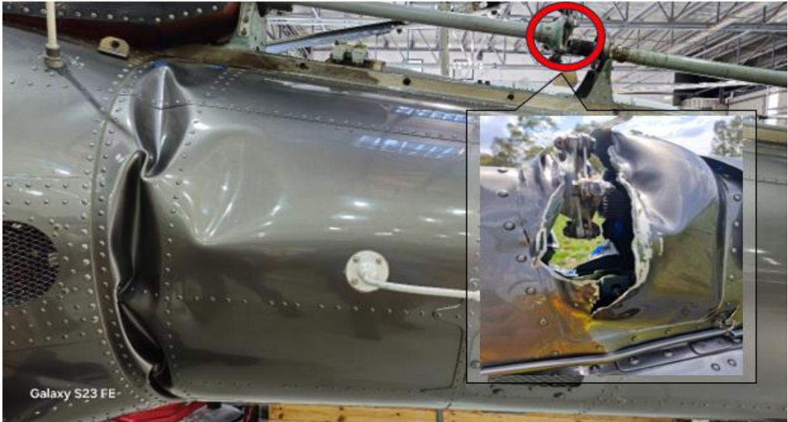
Figure 7: Damage to the tail boom attachment section and the decoupled tail rotor shaft. (Photo was taken after the helicopter was recovered).
