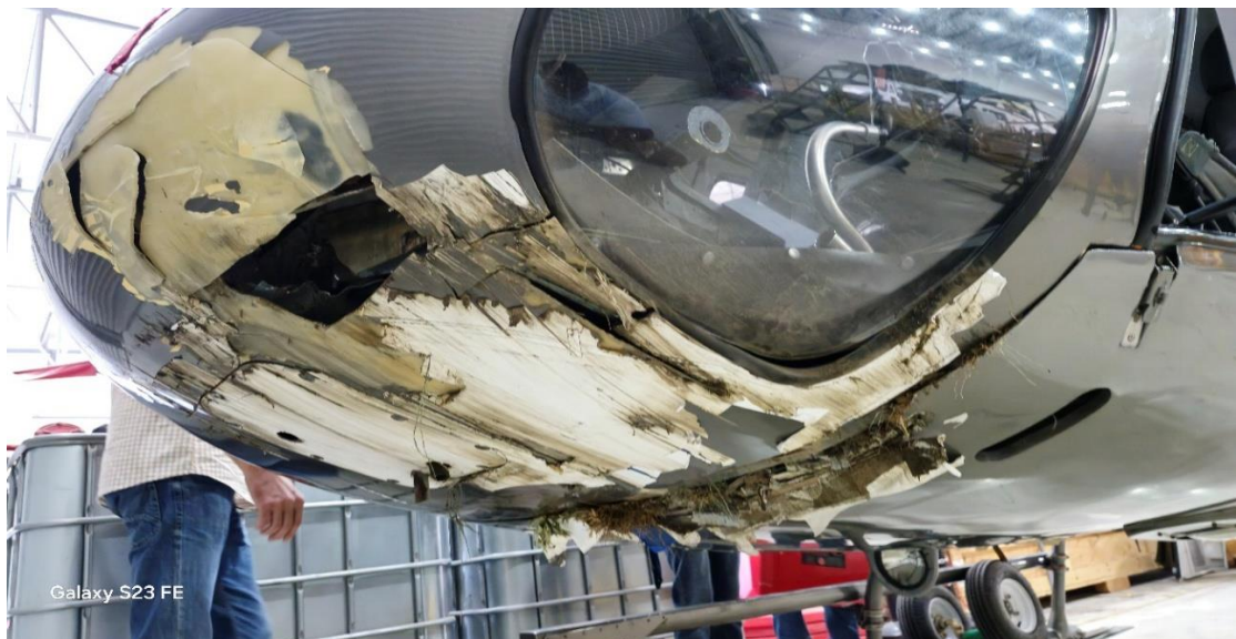
Figure 6: Damage to the bottom nose section.
