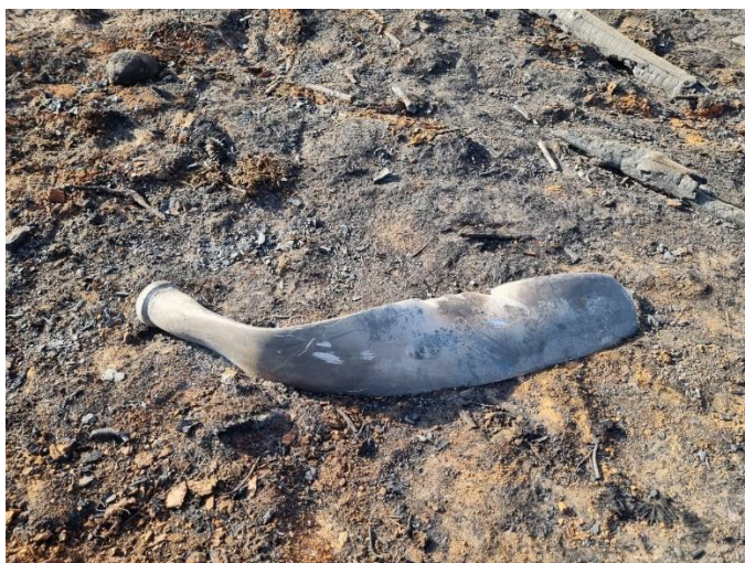
Figures 15, 16 and 17: Three of the five propeller blades that were recovered from the accident site.
