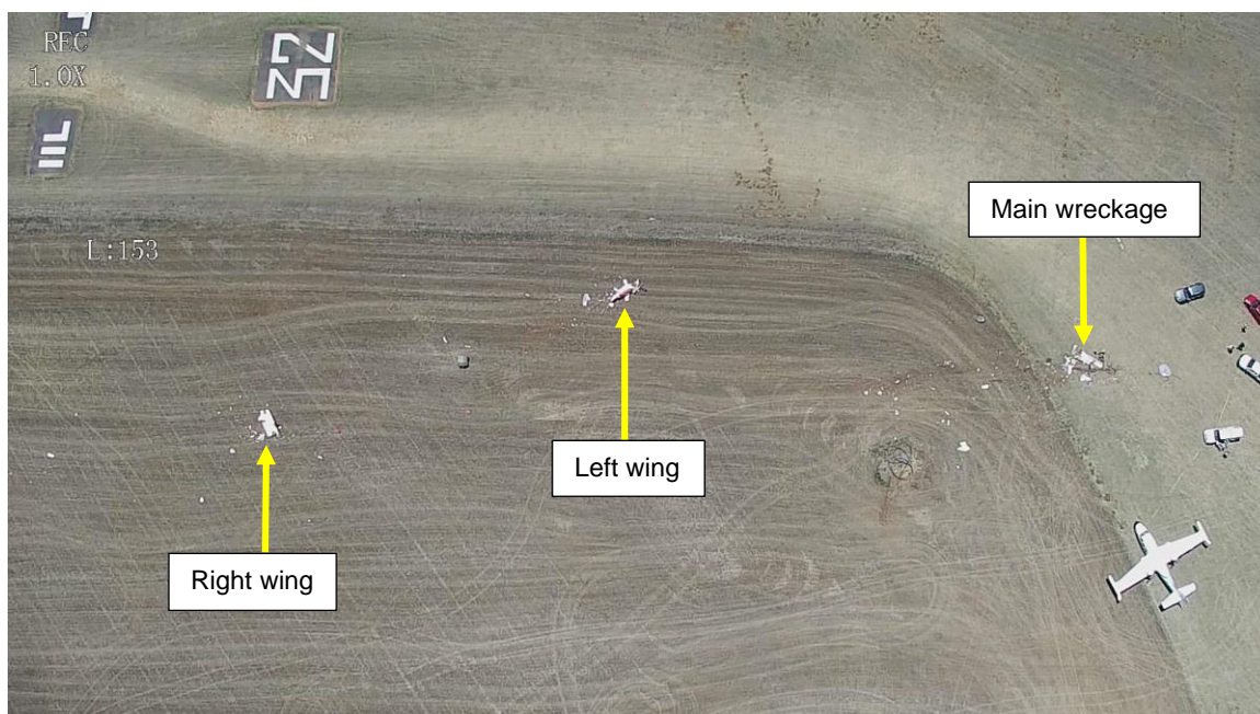
Figure 2: Drone camera footage depicting the wreckage distribution. (Source: Drone Ops)
