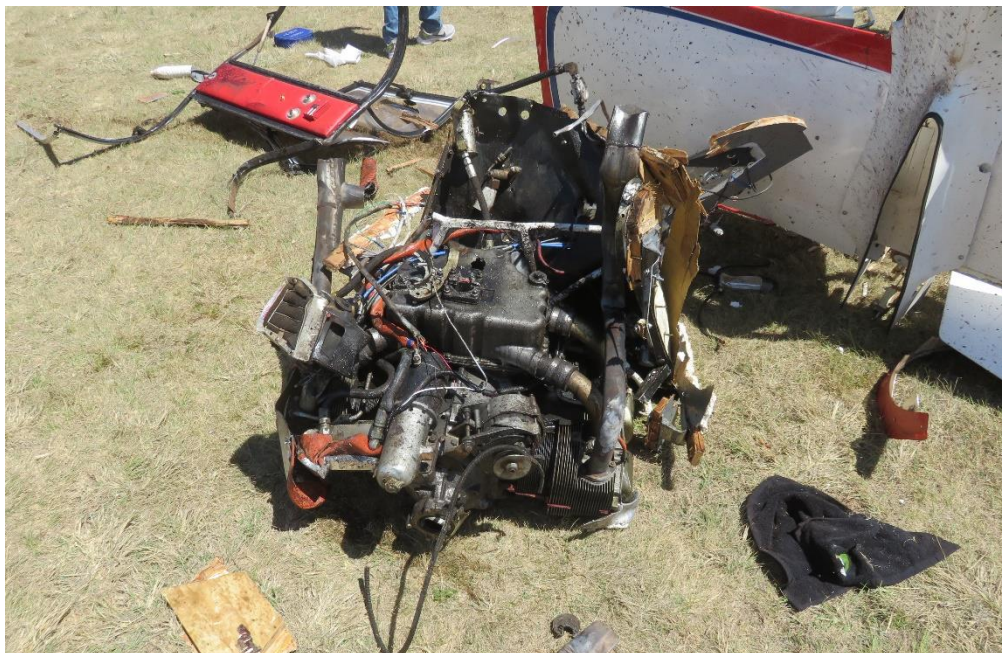
Figure 6: The engine in an inverted attitude with the propeller severed from the crankshaft.
