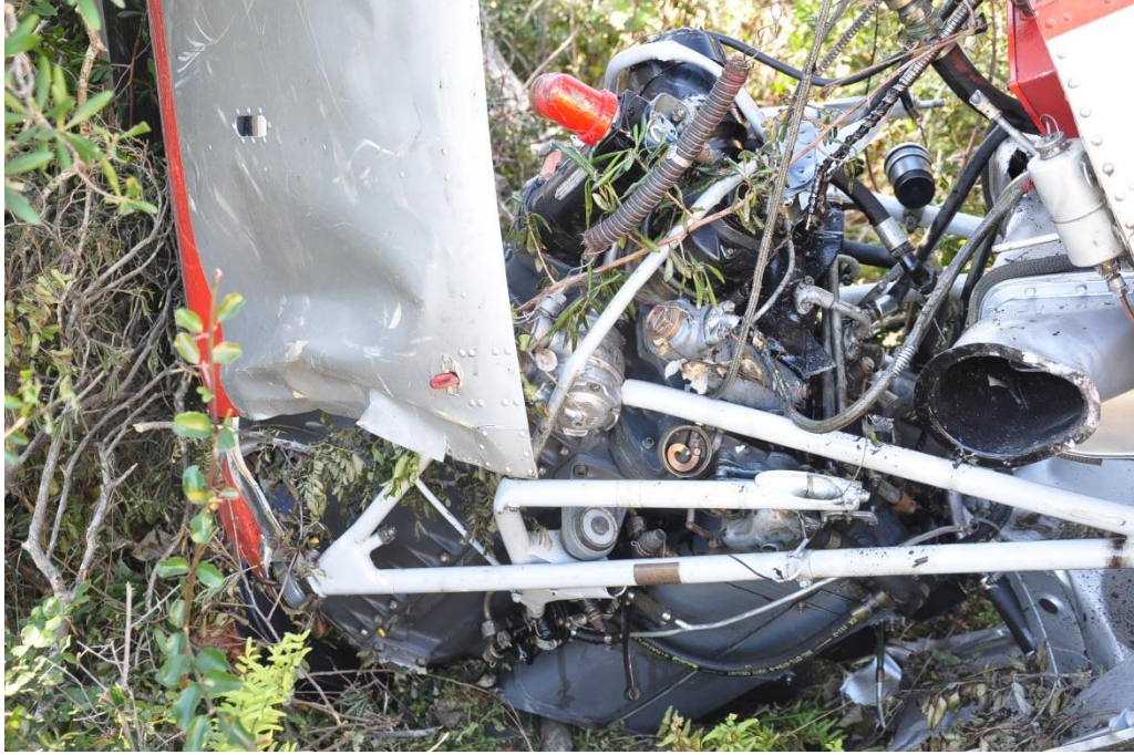
Figure 10: The engine did not separate completely from the aircraft.
