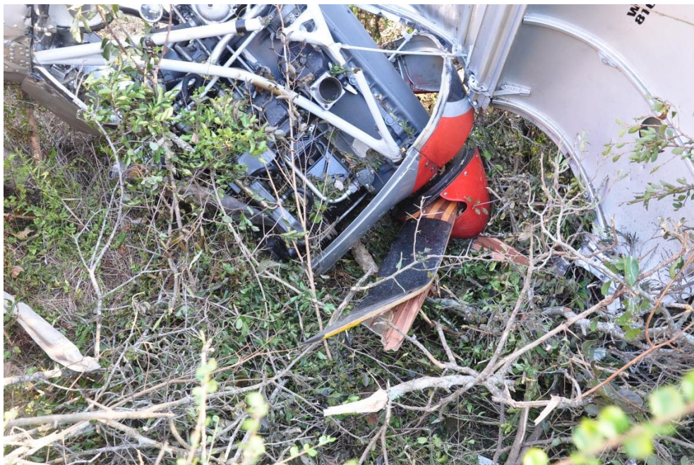
Figure 12: The piece of the propeller that remained attached to the spinner.
