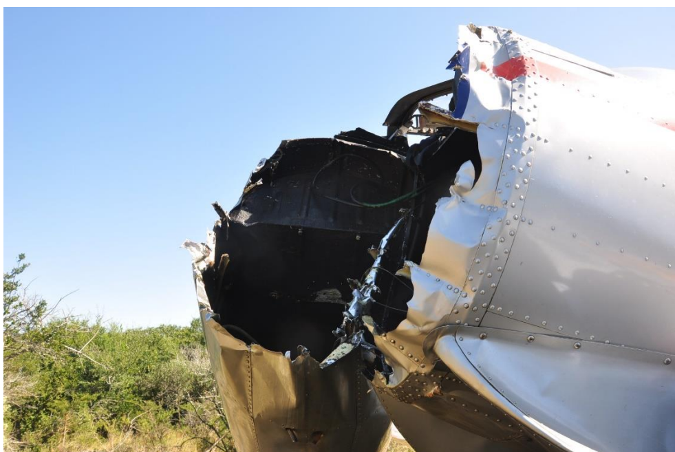
Figure 9. The torn empennage.
