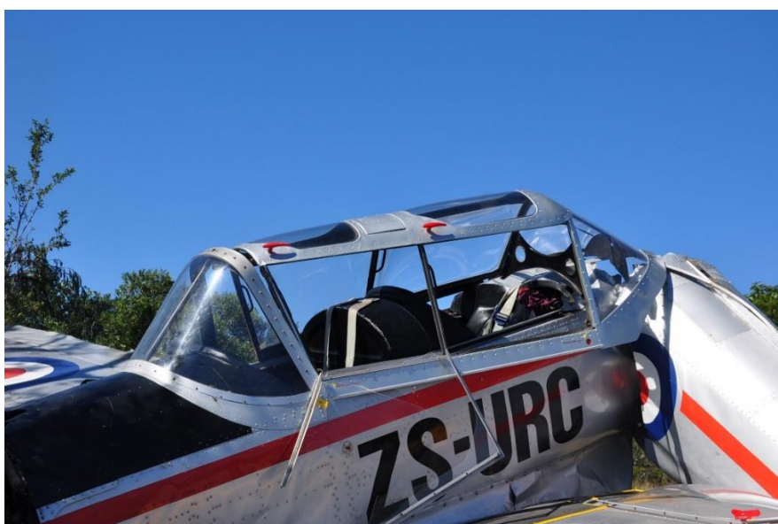
Figure 13: The canopy and fuselage were still intact with only the bent canopy rail.
