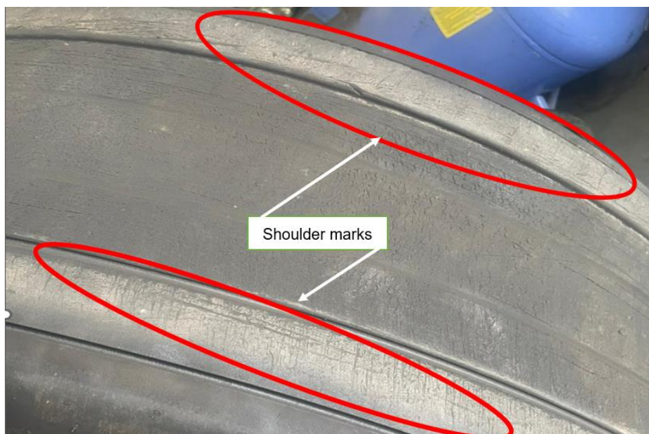
Figure 4: The shoulder marks on the Number 4 main tyre shoulder.
