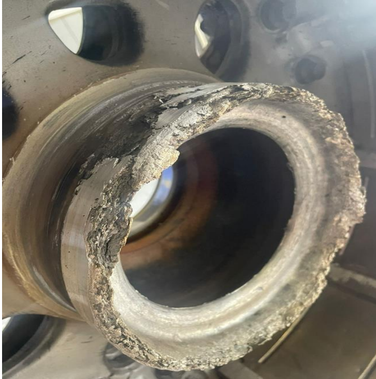
Figure 5: The fractured Number 4 hub.
