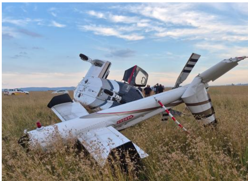
Figure 4: The helicopter with the broken tail boom.
