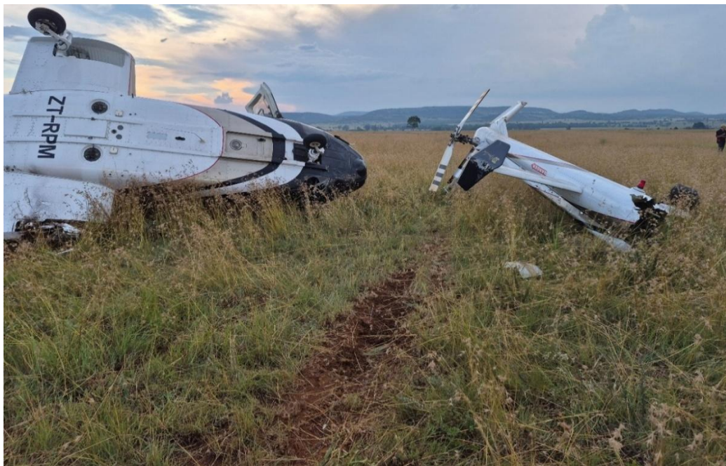
Figures 6: Witness marks impressed by the tail rotor.
