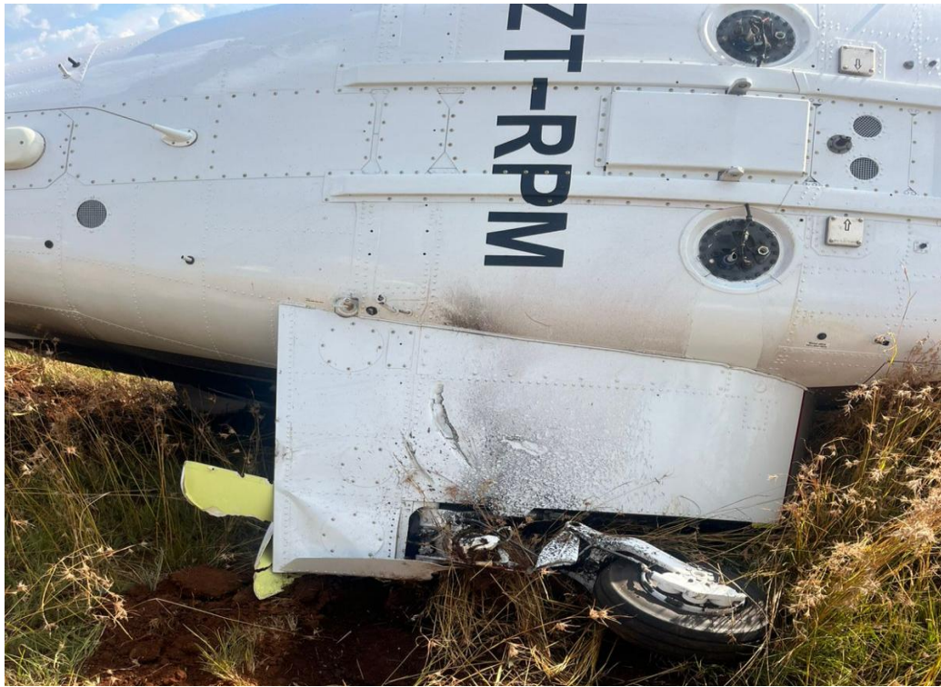
Figure 5: The damaged left main wheel.
