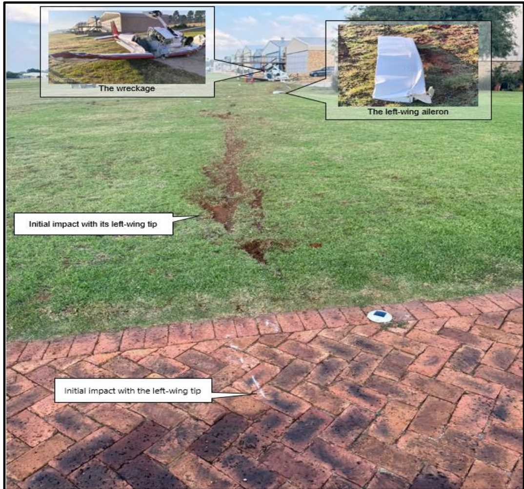
Figure 7: Wreckage impact marks and distribution.
