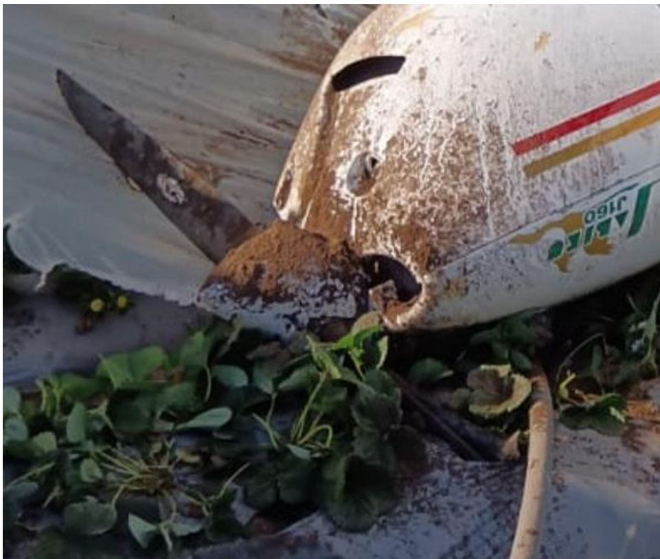
Figure 7: The position of the propeller indicates that the engine was not turning when it impacted the ground. (Source: Pilot)
