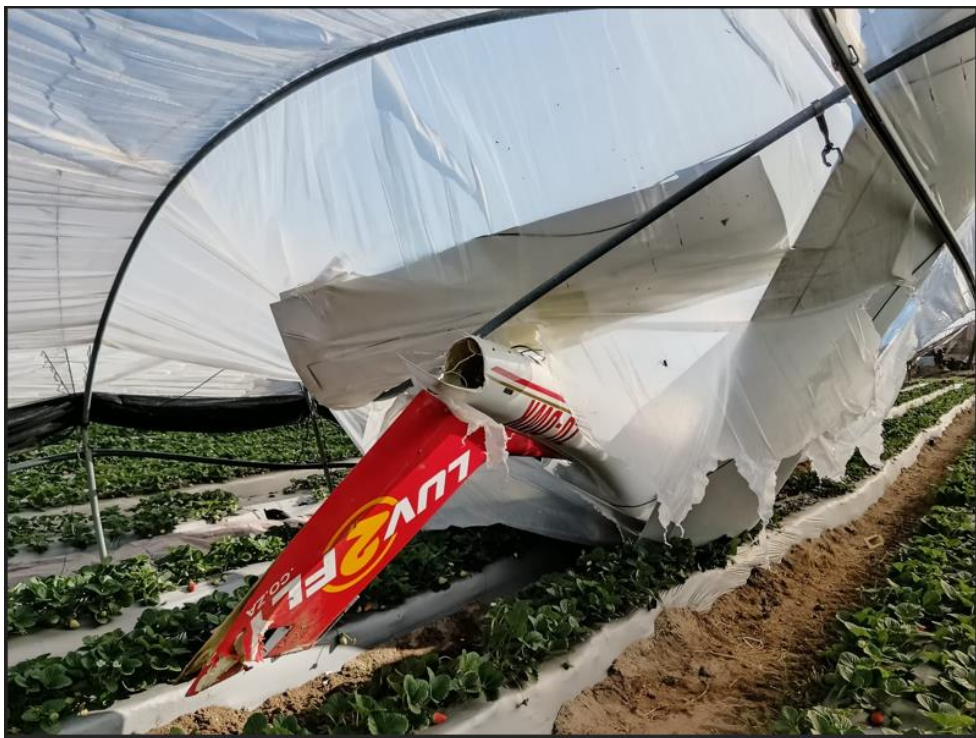
Figure 6: The damaged vertical and horizontal stabilisers. (Source: Pilot)
