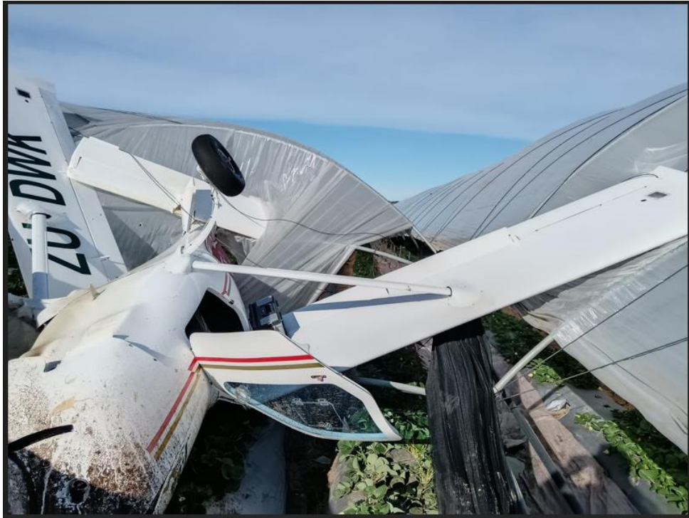
Figure 5: The damaged fuselage and wings. (Source: Pilot)
