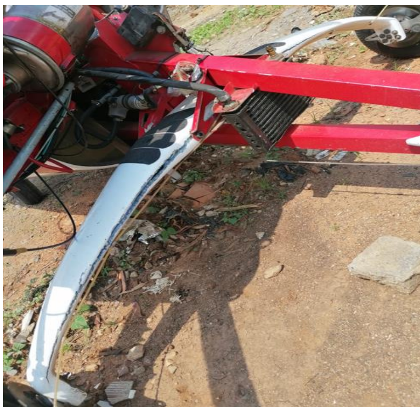
Figure 4: The landing gear strut.
