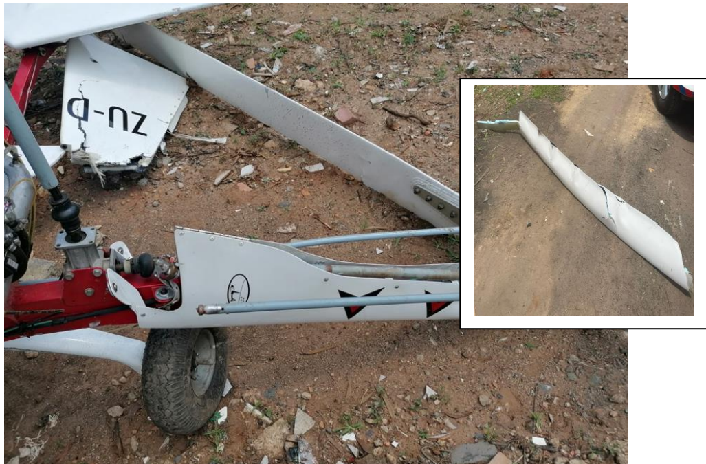
Figure 6: The main rotor mast and (inset) the severed blade.
