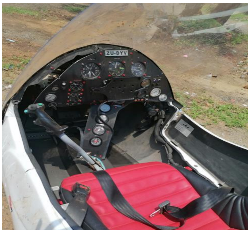
Figure 6: the instrument panel.
