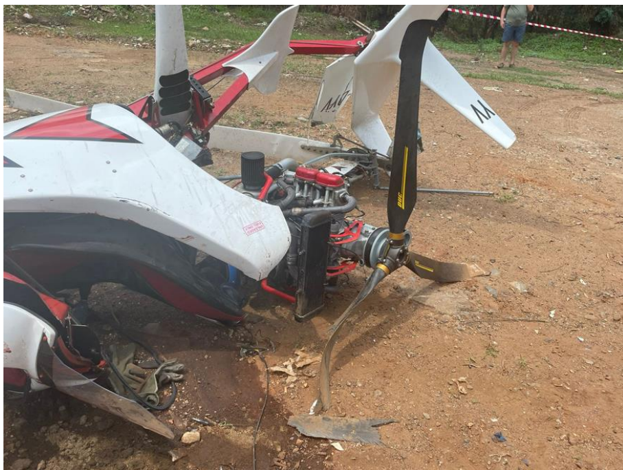
Figure 7: The damaged propeller blades.
