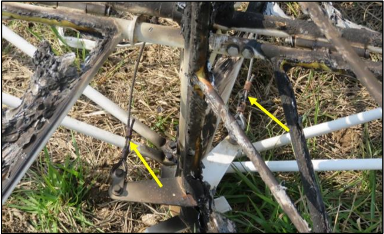
Figure 7: The two rudder cables were secured on both sides of the rudder attachments.
