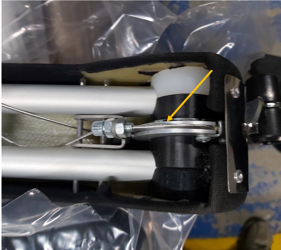
Figure 4: New pulley made of aluminium (sealed item before installation on the aircraft).
