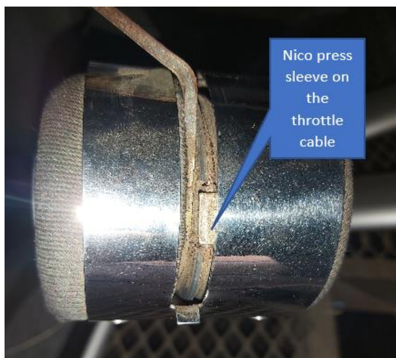
Figure 3: Throttle showing Nico press sleeve on the cable.
