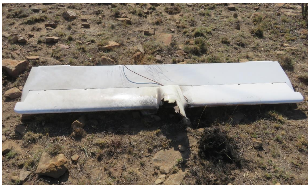
Figure 8: The horizontal plane with the vertical fin ripped off.
