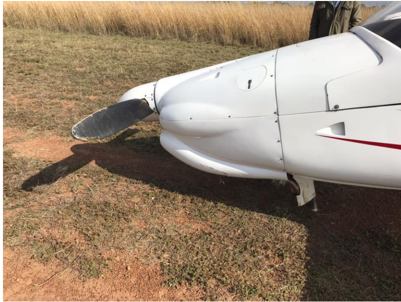
Figure 3: One of the damaged propeller blades. (Source: Pilot)
