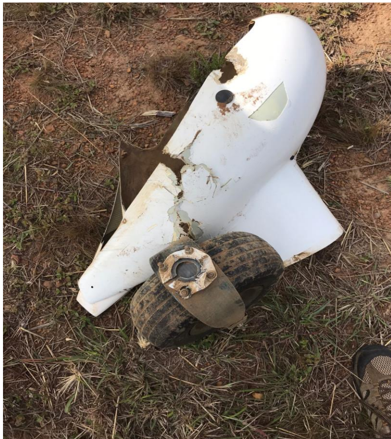
Figure 4: The nose wheel separated from the wheel strut. (Source: Pilot)
