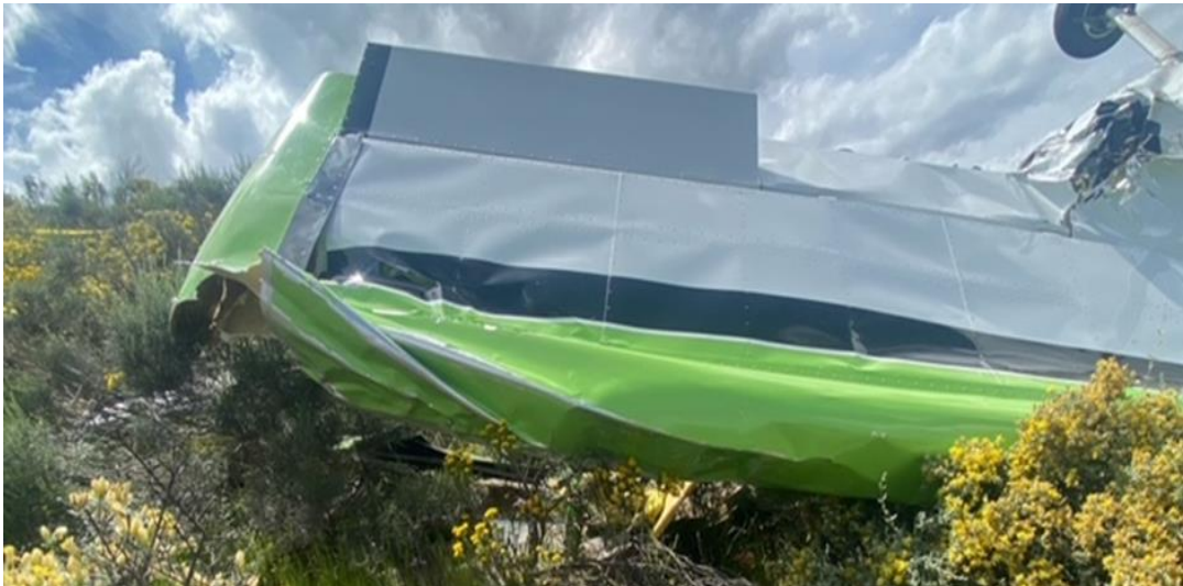
Figure 5: The damaged right-wing tip.
