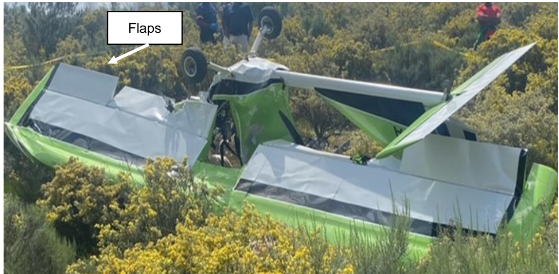
Figure 6: The damaged wings.
