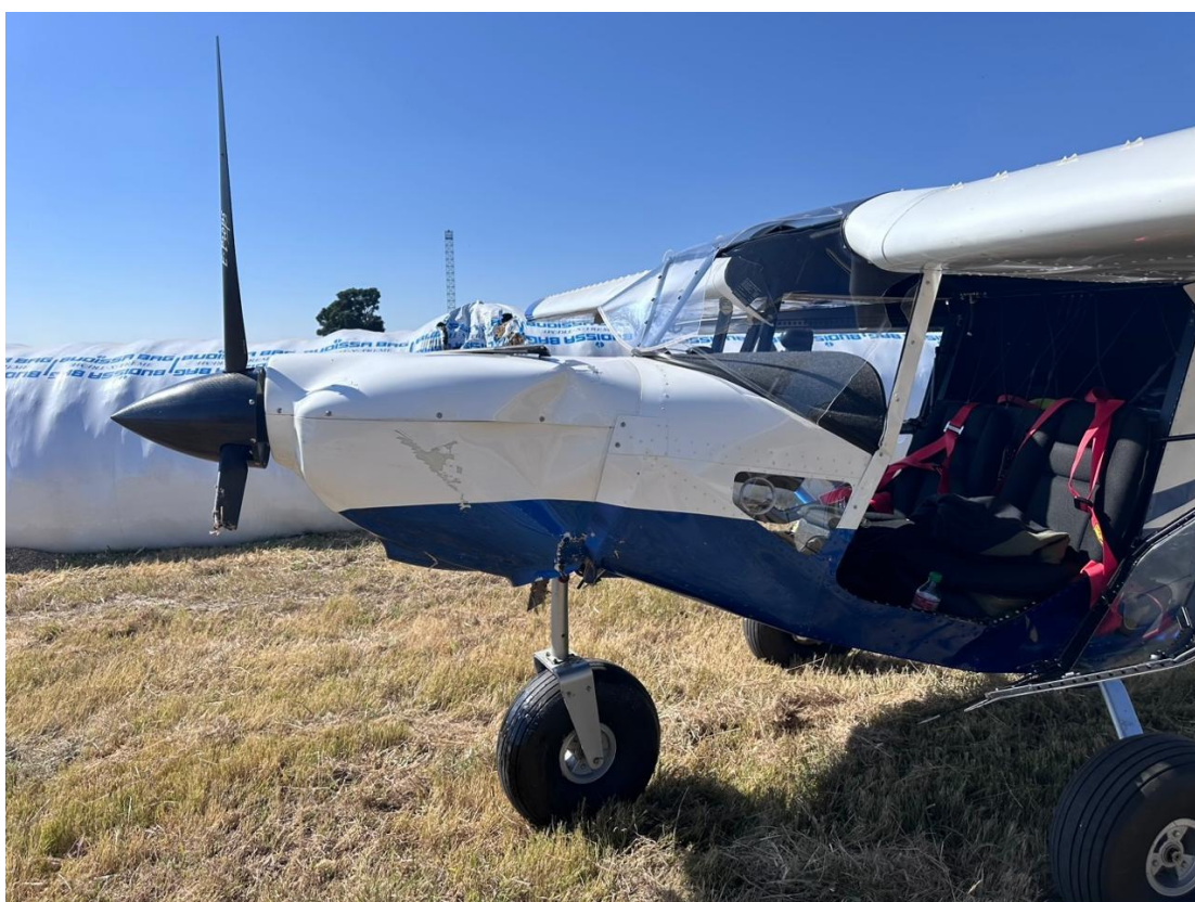
Figure 3: The aircraft post-accident with the damaged propeller blades and nose section. The silage bag is in the background.
