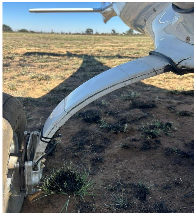
Figure 4: The aircraft's right main wheel strut had a crack. (Source: Pilot)
