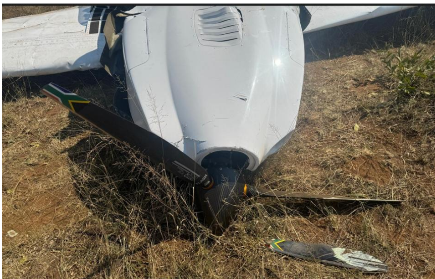
Figure 9: The propeller with one broken blade; the other two blades had remained intact.
