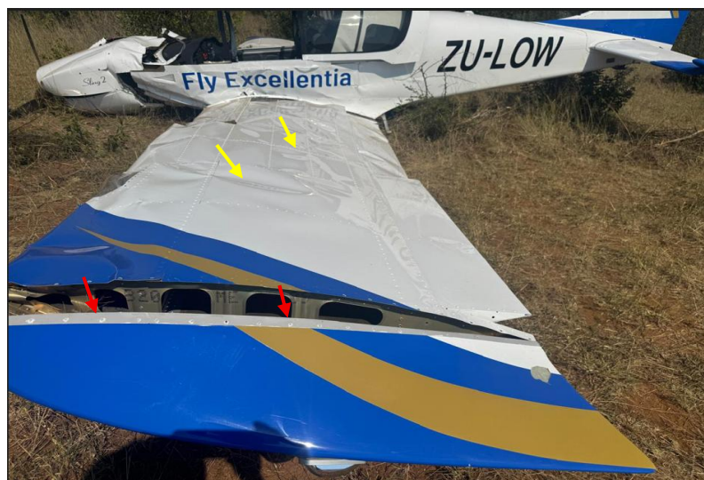
Figure 6: Evidence of buckling (yellow arrows) on the left wing and the rivets that sheared off (red arrows), resulting in the separation of the wing fairing.
