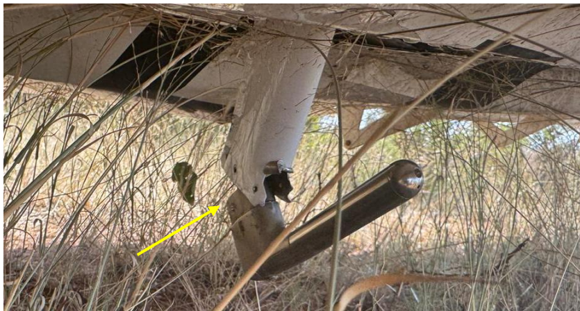
Figure 5: The broken pitot tube.
