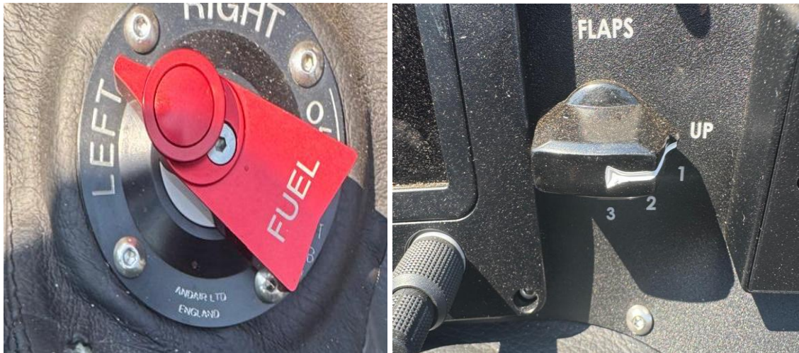
Figures 7 and 8: The fuel selector on the left tank (left picture). The flap control switch in the UP position (right picture).
