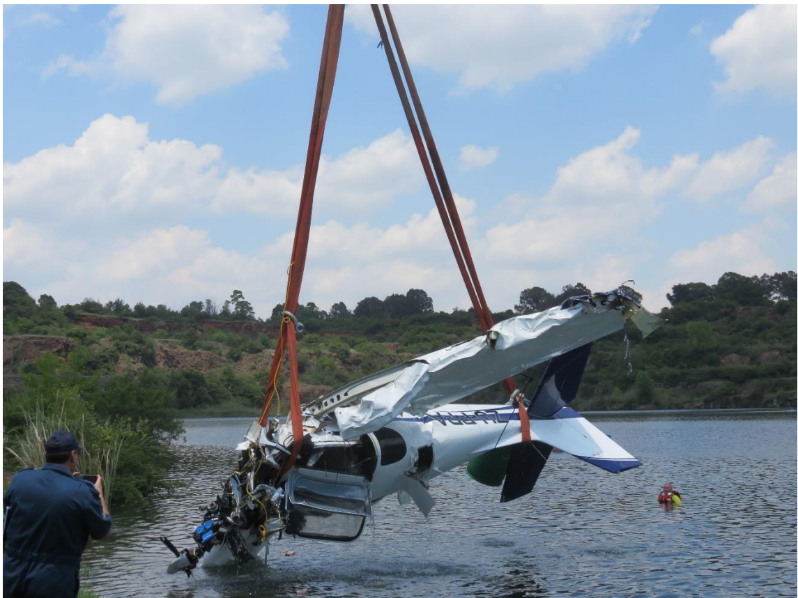
Figure 6: Wreckage being lifted from the water by a crane.
