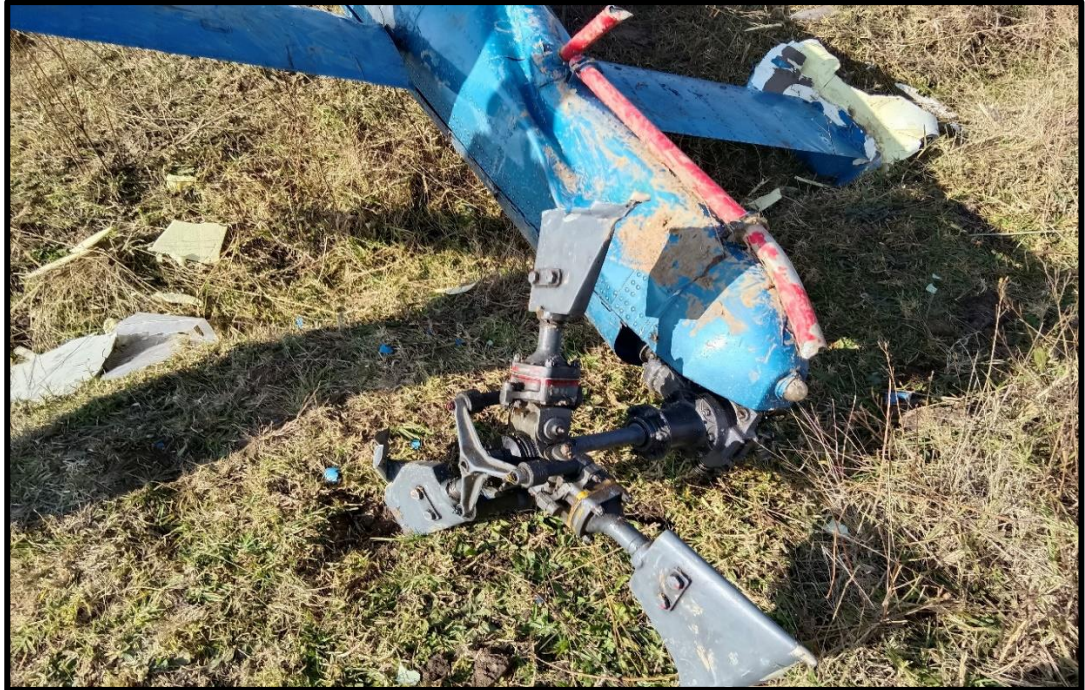
Figure 7: The damaged tail rotor.
