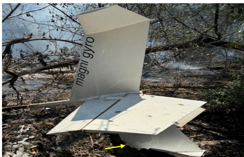
Figure 5: The tail section and the damaged left fin/horizontal stabiliser.
