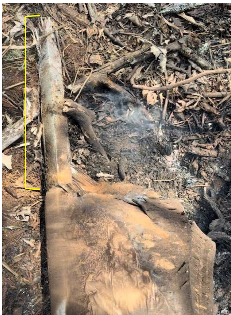
Figure 9: The severed tip of the main rotor blade that hit the tree branch.
