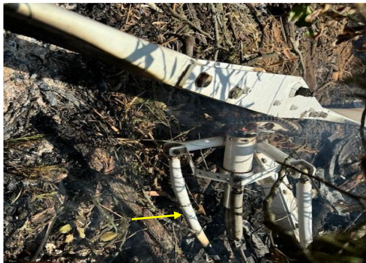
Figure 10: The main rotor head and the bent rod.
