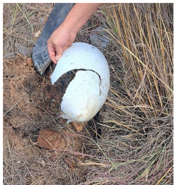
Figure 5: The cracked aircraft spinner.
