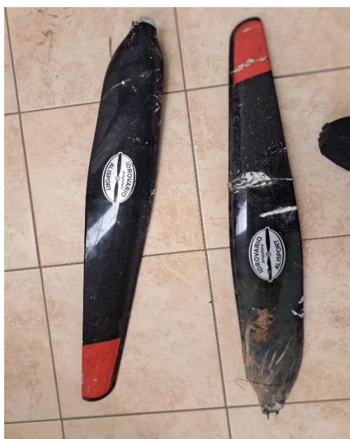
Figure 4: The damaged propellers.
