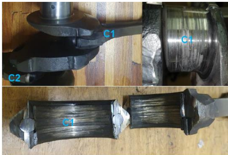
Photo 9: Connecting rod C1 condition (Digital)
