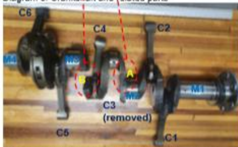
Photo 6: Position of primary fractures A and B and other parts (Digital)
