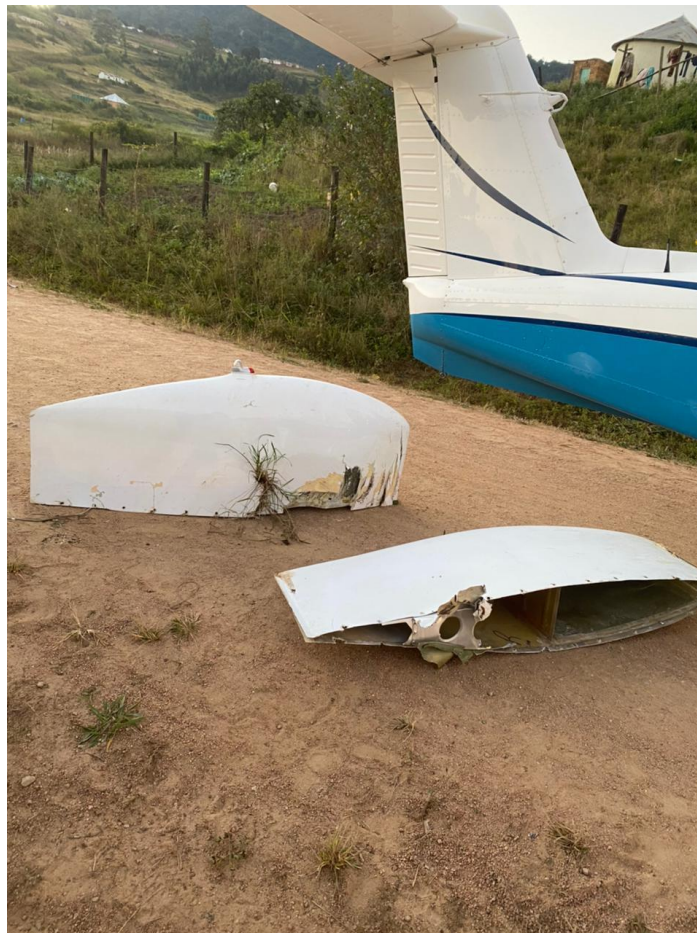
Figure 7: The severed left- and right-side wing tips. (Source: Pilot)
