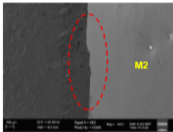
Fractograph 1: Fracture A, surface morphology (145X, SE, 20kV, FEGSEM)
