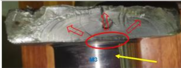
Photo 8: Fracture B, surface geometry (Digital)
