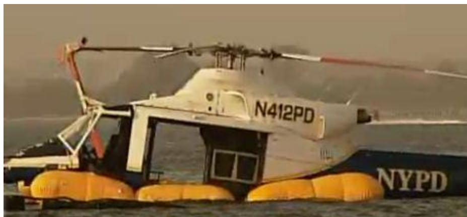
Figure 1: A helicopter fitted with floatation devices. (Source: New York Police Department website)
