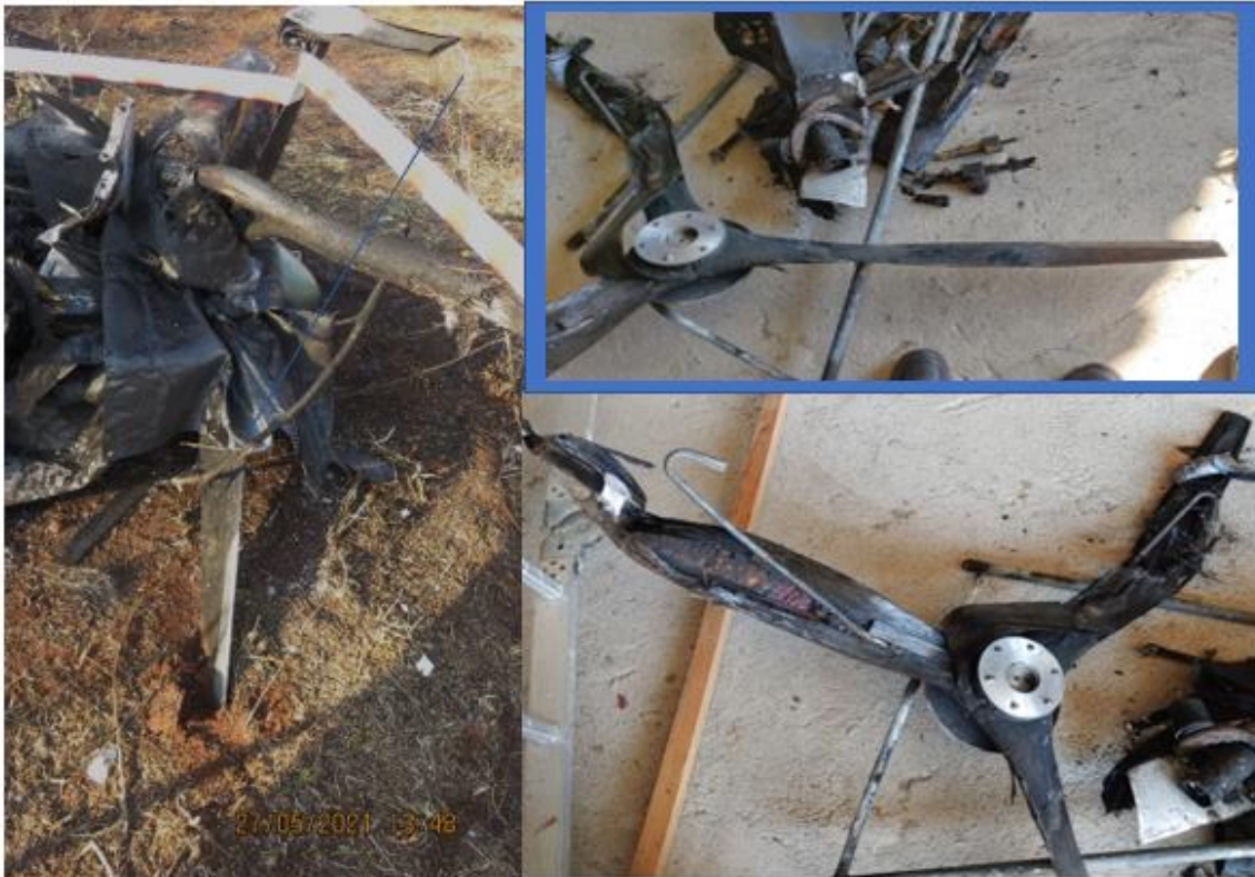
Figure 5: The damage on the propeller blades.
