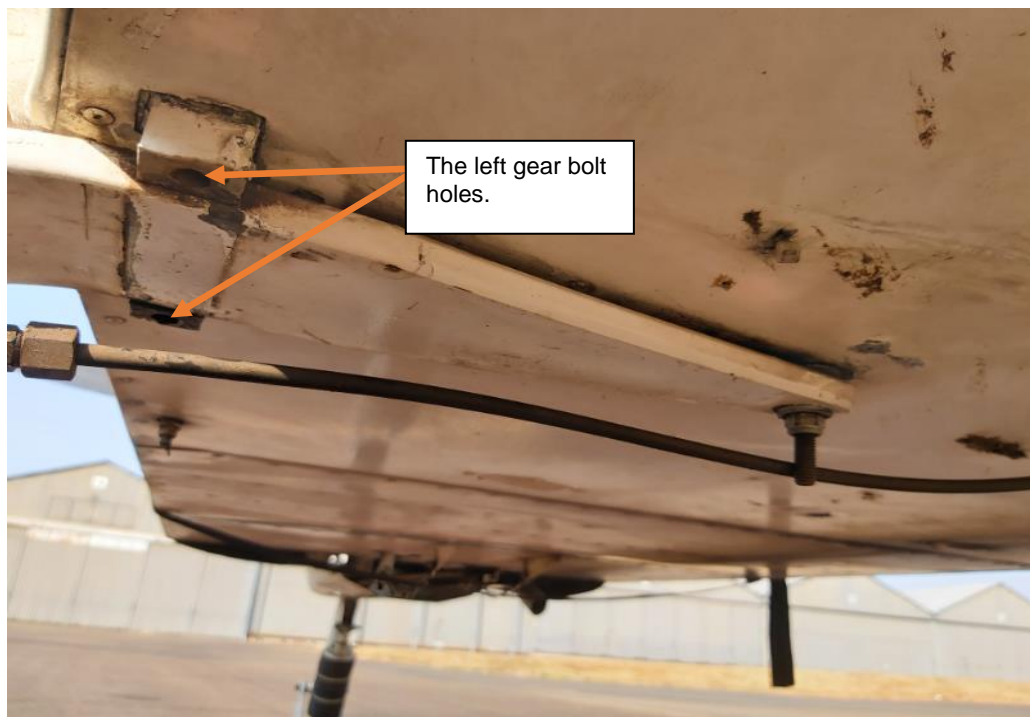
Figure 4: The left landing gear attachment area.
