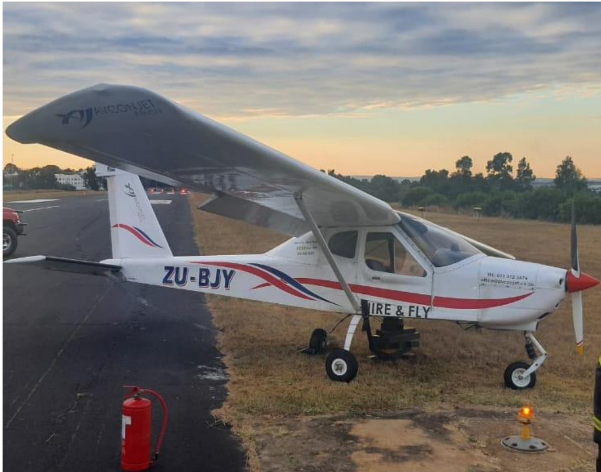
Figure 2: The aircraft post-accident with the damaged left gear.
