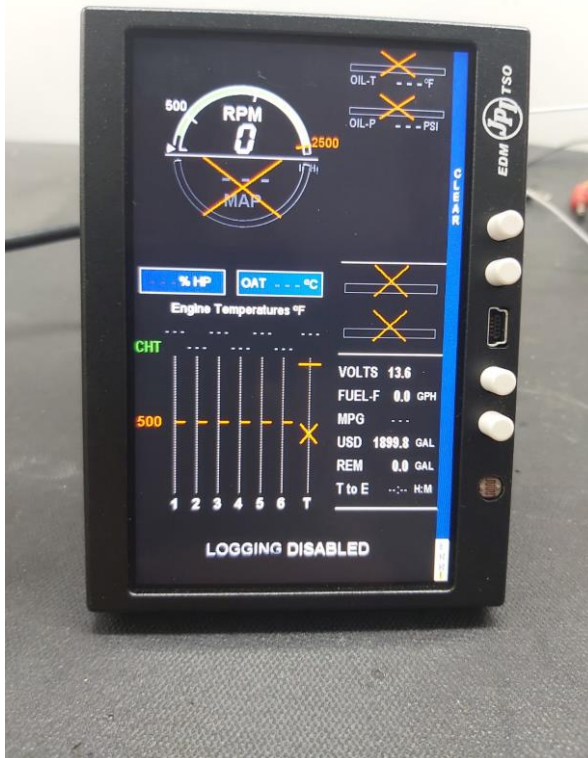
Figure 3: Picture of the JPI instrument which monitors engine parameters. (Source: Pilot)
