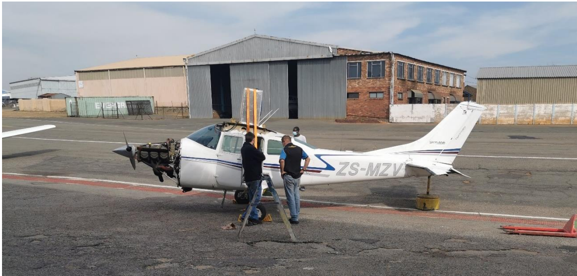
Figure 10: The engine ground run following recovery of the aircraft.
