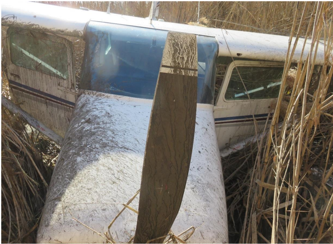
Figure 9: The front view of the aircraft with one of the propeller blades slightly bent.
