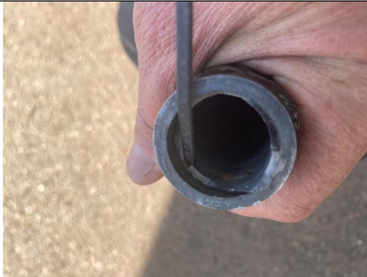
Figure 3: The area on the front-side of the nose gear strut where the crack initiated.
