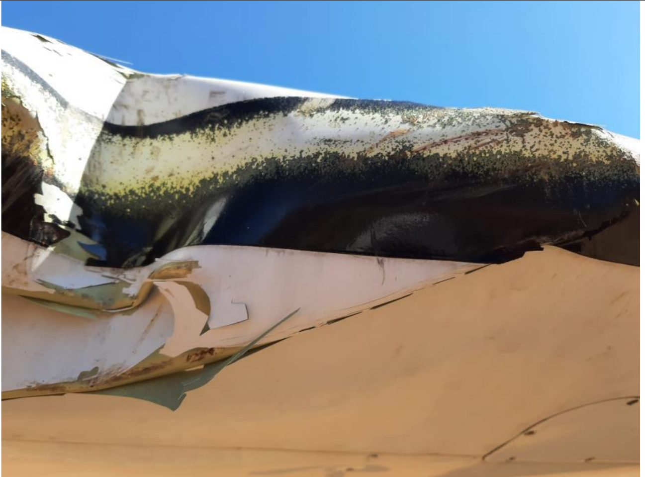
Figure 2: Damage on the right wing tip. (Source: Operator)
