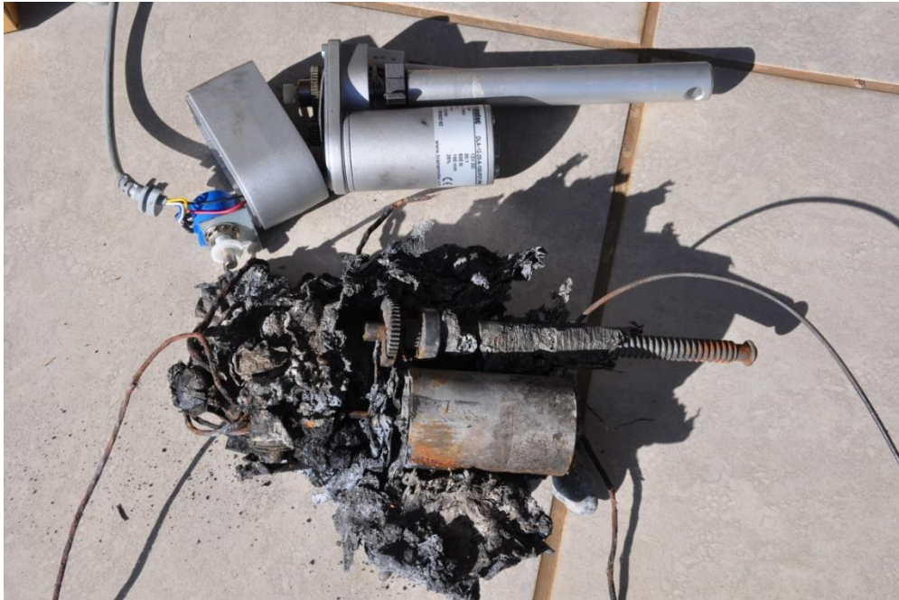
Figure 13: A serviceable flap motor in the retracted configuration (top); and a fire damaged flap motor in the retracted configuration (bottom).
