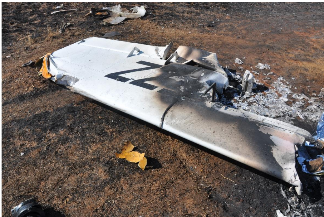
Figure 11: The left-wing with impact damage on the wing tip.
