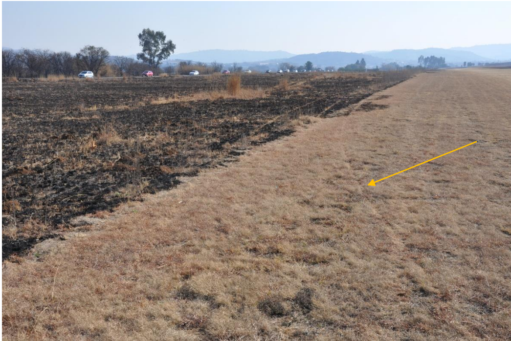
Figure 8: Wheel markings of where the aircraft started to veer off to the left.
