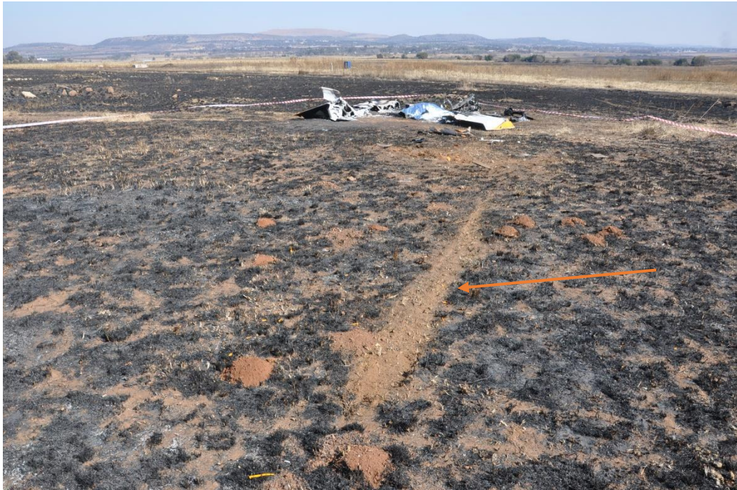
Figure 10: First ground marking after the left wing contacted the ground.
