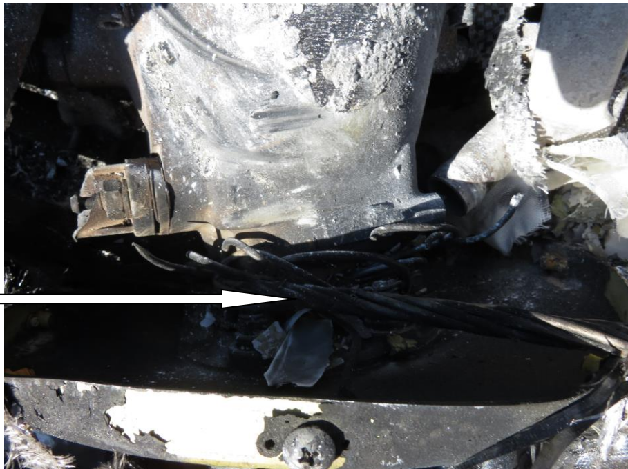
Figure 1: Powerline cable entangled around the propeller flange.
