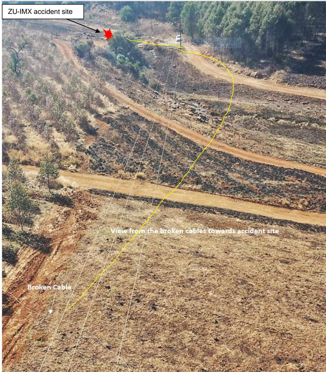
Figure 4: Aerial view of ZU-IMX flight path in yellow; as well as the severed powerline cable the aircraft collided with, and view of the accident site.
