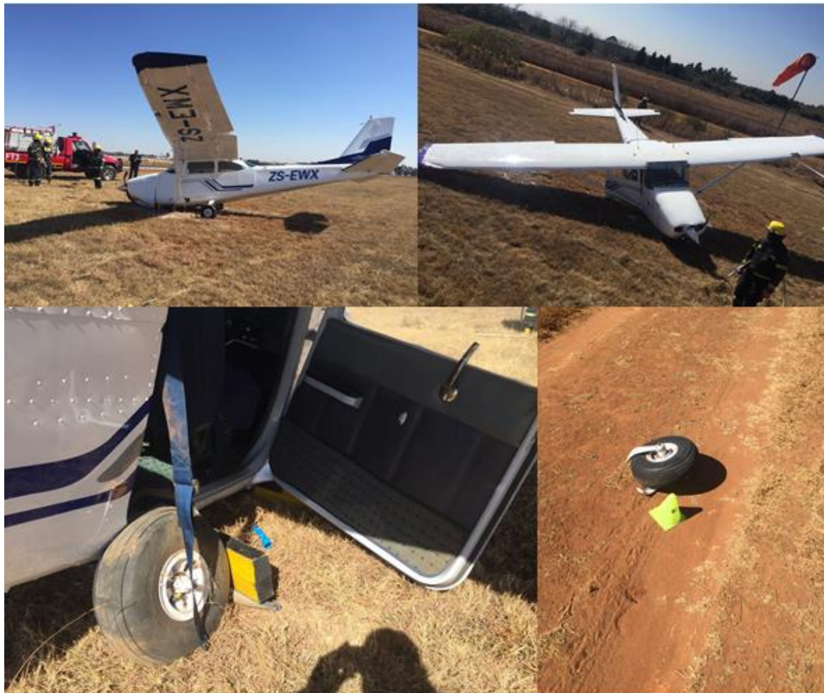
Figure 1: The accident aircraft with damages sustained during the accident sequence.
