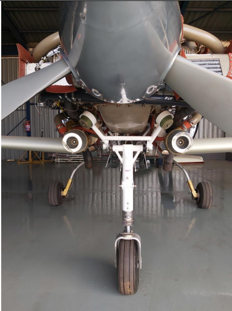
Figure 4: Repaired nose wheel assembly.
