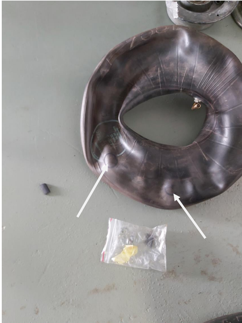
Figure 2: The tyre tube with white arrows showing the two punctures.
