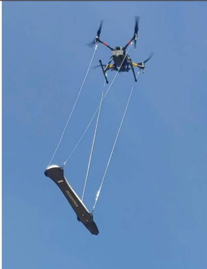
Figure 3: This is how the payload was suspended on the drone. (Source: geometrics.com)
