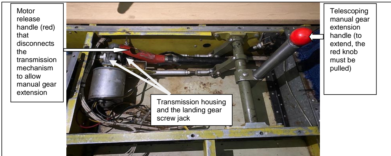
Figure 4: The landing gear manual extension lever in an extended position.
