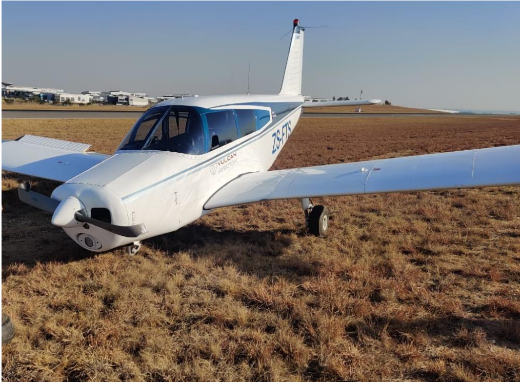
Figure 1: The aircraft post-accident showing the damaged propeller and broken nose gear. The photo was taken after the aircraft was moved from the runway. (Source: Pilot)
