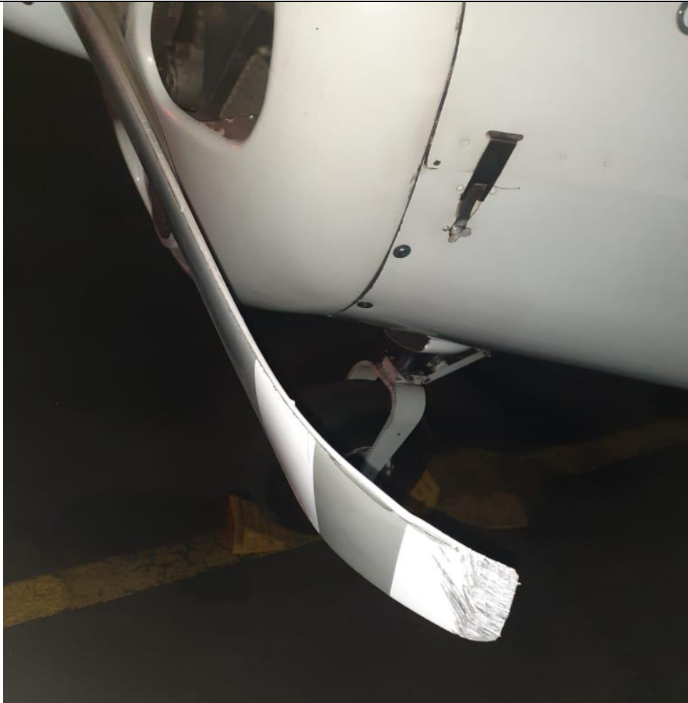
Figure 4: The damaged propeller.
