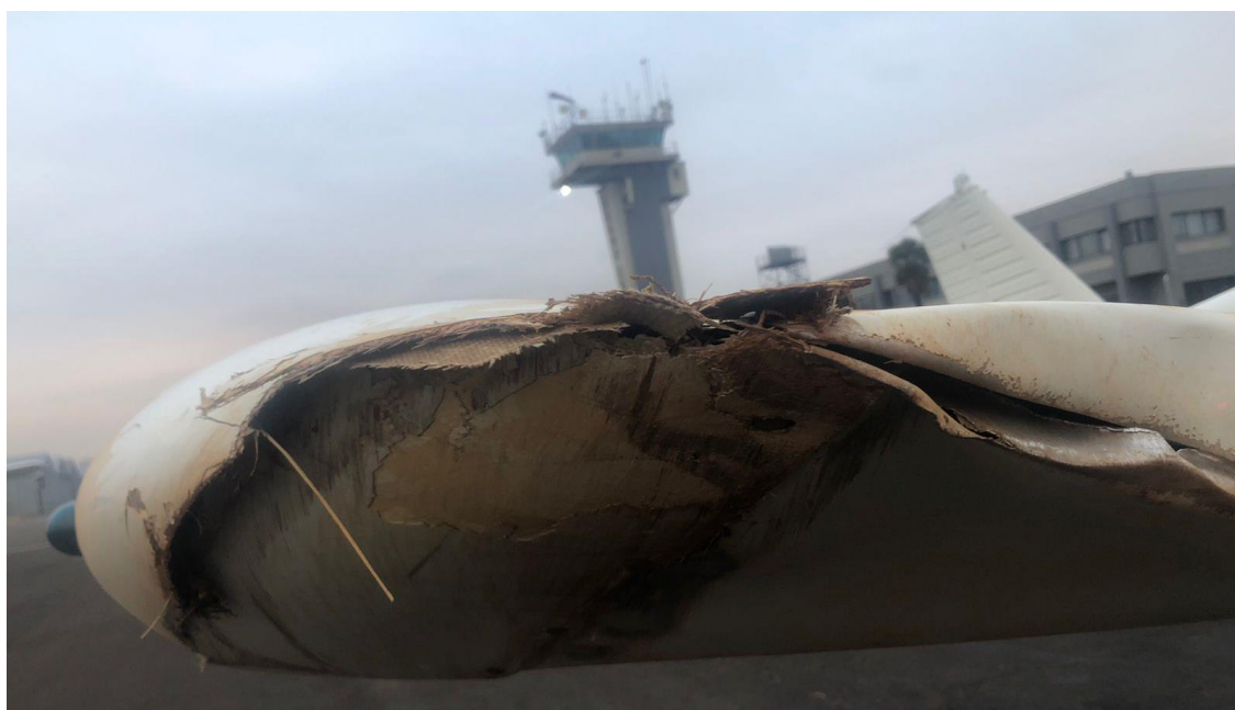
Figure 3: Damage to the right-side wing tip.
