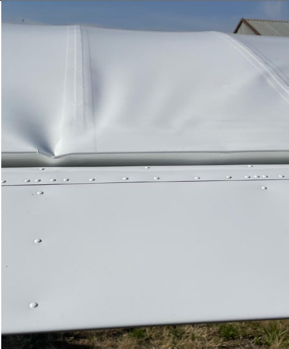
Figure 2: Damage to the trailing edge. (Source: Pilot)
