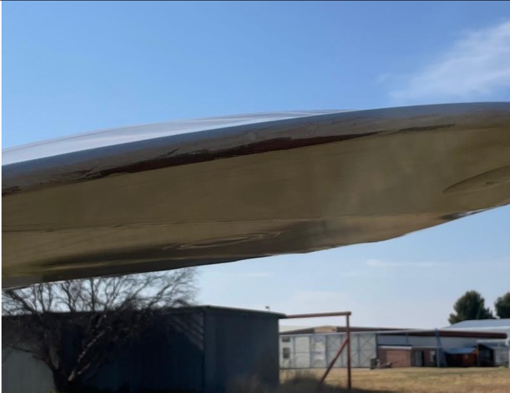
Figure 1: Damage to the leading edge. (Source: Pilot)
