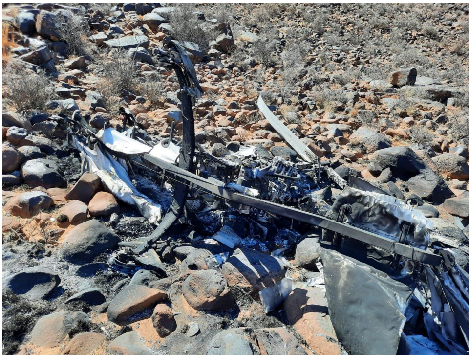
Figure 4: The burnt gyrocopter laying on its right-side at the accident site. (Source: Pilot)
