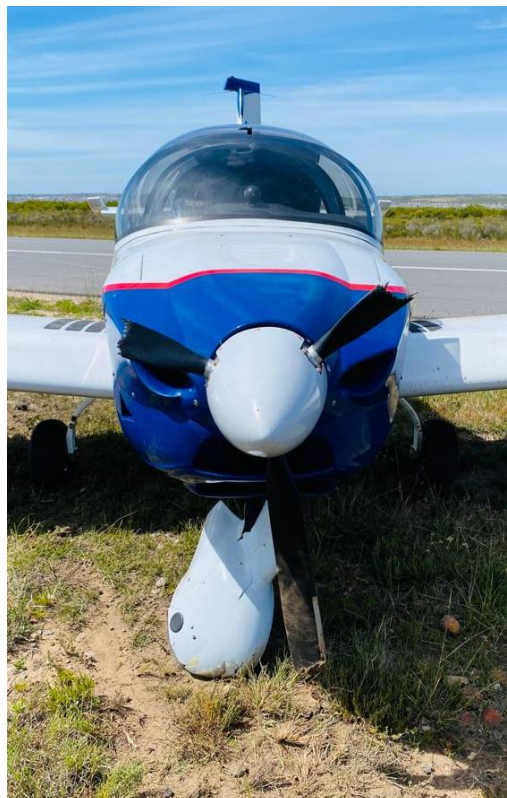
Figure 2: Front view of the aircraft showing damage to the propeller and nose landing gear. (Source: Pilot)
