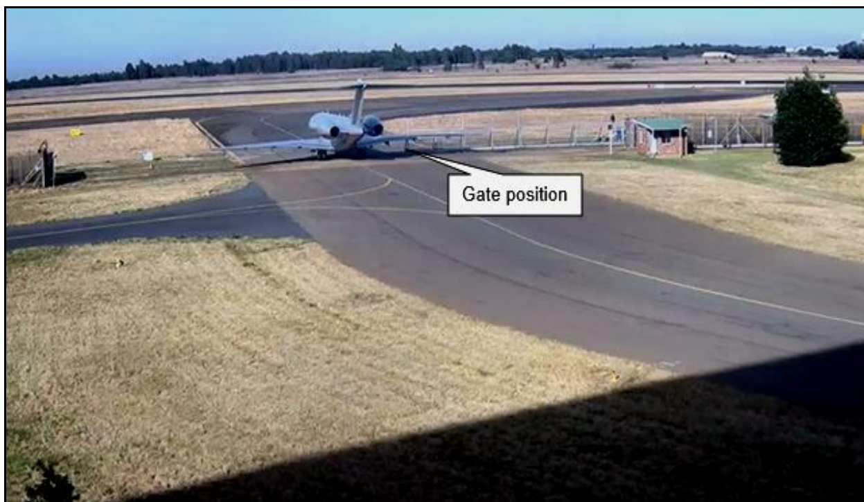
Figure 9: In this screenshot, the gate stops moving after colliding with the right wing leading slat.
