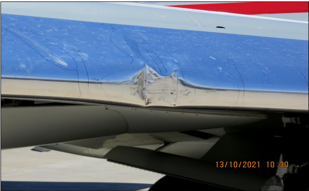
Figure 3: Deformation of the number 2 leading-edge slat on the right wing.
