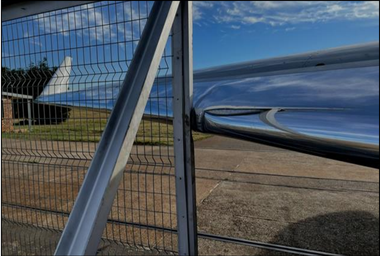
Figure 10: The gate whilst in contact with the leading-edge slat. (Source: Fireblade Aviation)
