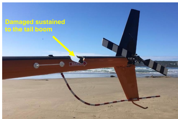
Figure 2: The severed tailboom skin. (Source: Operator)
