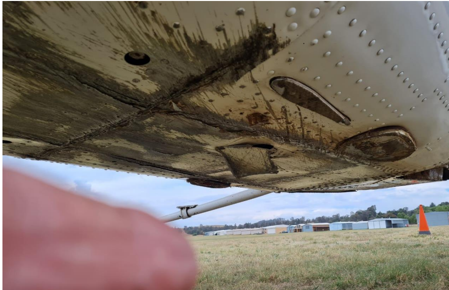
Figure 3: The damaged underbelly of the aircraft. (Source: Pilot)
